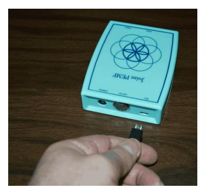
Make sure the MR72 is OFF and plug the Mini-USB cable into the mini-USB jack in the unit. The MR72 is OFF if the green LED ring light is not lit.
